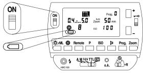
Fig. 3: The battery warning indicator
